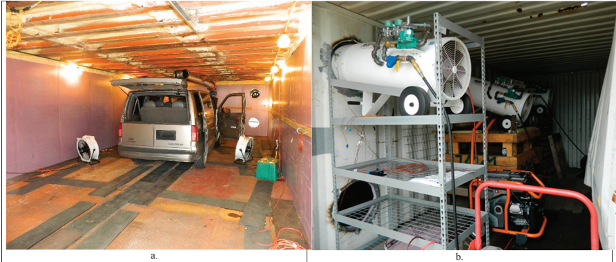
Fig. 1. (a) Vehicle used for experiments parked inside a container heat treatment facility constructed by Willenius Wilhelmsen Logistics (WWL), and (b) the 500,000 BTU propane heaters used to generate lethal temperature extremes greater than 60°C for heat treatment of vehicles.
